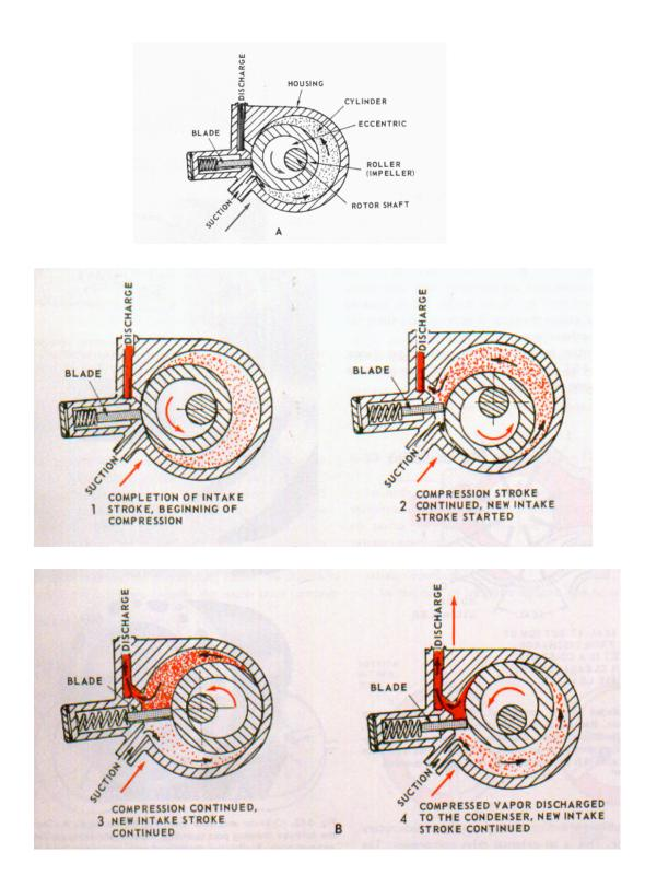
tolerant for the presence of liquid refrigerant and the high working temperature helps to make the compressor more resistant against a floodback (More about this in the next chapter).
