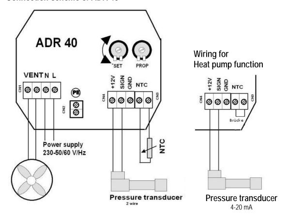
The scheme above shows the connection of a pressure transducer and alternatively the connection with a NTC sensor.
